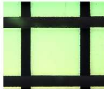
Borosilicate substrate diced at 1mm / sec
